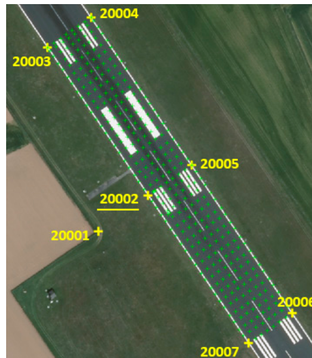
Figure 1. Basic (zero) geodetic net and GRID on the runway.
